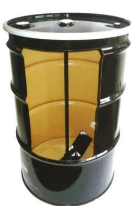
The nylon G1.5 Tri-Sure® Agitator plug features the patented R-plug™ retention ring which helps hold the plug gasket in place during opening & closing. The R-plug™ design also lowers the opportunity for gasket looping during tightening and the potential for crimped gasket leakage. The Tri-Sure® agitator plug works with marketplace industry standard wrenches.
