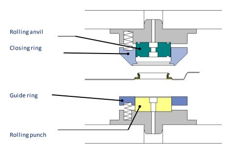
In the **2nd operation** die the flange is placed on the rolling punch and is located by the guide ring
