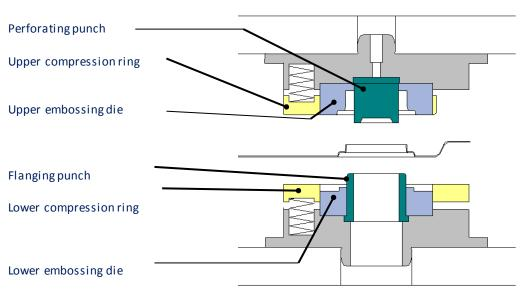
In the **1<sup>st</sup> operation** die a cylindrical blank is punched out of the end- material with the perforating punch and the flanging punch.
