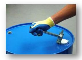
To remove the metal Tab-Seal cap, use the Tri-Sure universal plug wrench. Place the pin of the plug wrench in the hole of one of the ears and pull the tool gently backwards. Rock the tool from side to side, so that the beginning of the two score lines open up. Now pull the tool backwards and use the leverage of the tool to fully break away the centre strip of the Tab-Seal cap.
