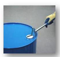
To place the pin of the tool in the hole in the ear, the ear may have to be raised above the surface of the drum Use the flat side, provided in the handle of the plug wrench to do this.
