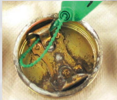
Chromium 6 passivation: result 240 hour neutral salt spray test
