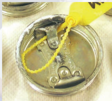
Chromium 3 passivation: result 240 hour neutral salt spray test
